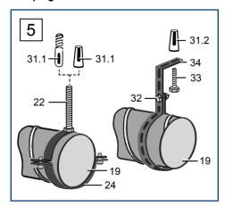
Ensure a spacing of max. 1.5 m between the duct attachments [23].
