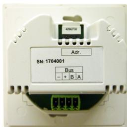
The connection of a wired external sensor, takes place on the RS 485 interface of the RLS 45 O/K control (max. 3 sensors per control).
